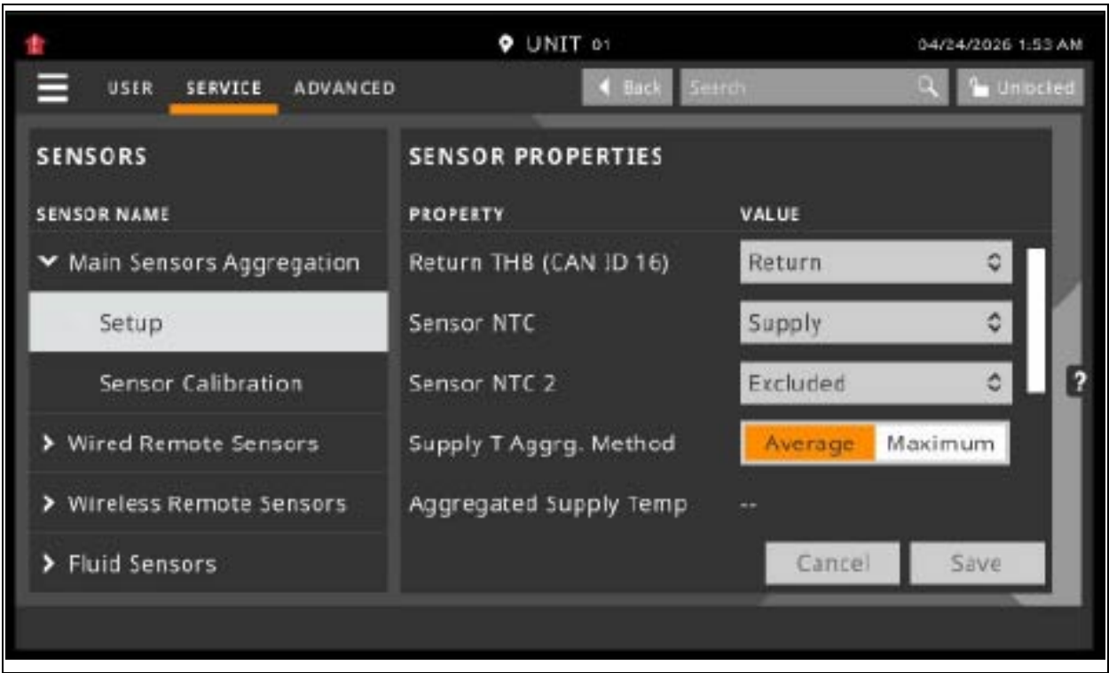
Figure 3.7 Enabling Supply Sensor Aggregation
